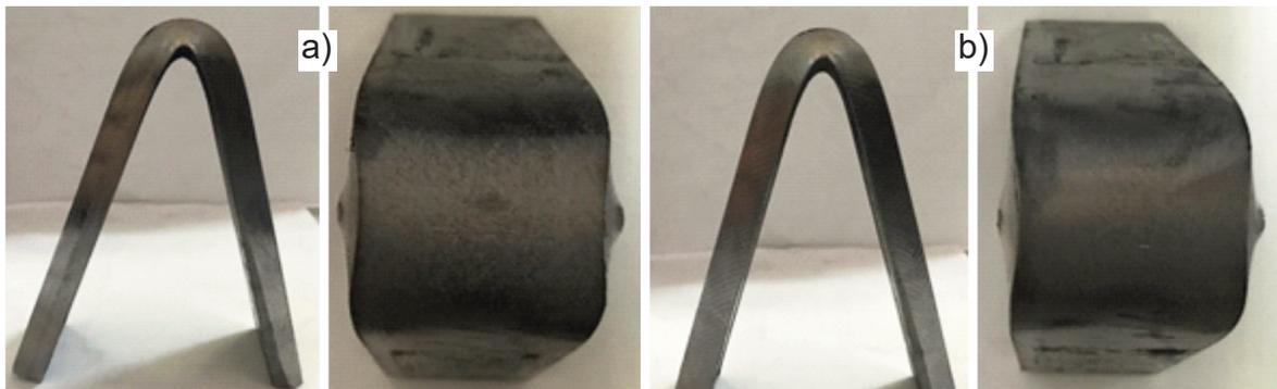
Figure 4. Side and top view of the bent specimens of 10 mm thick S3 (a) and S4 (b) strips
