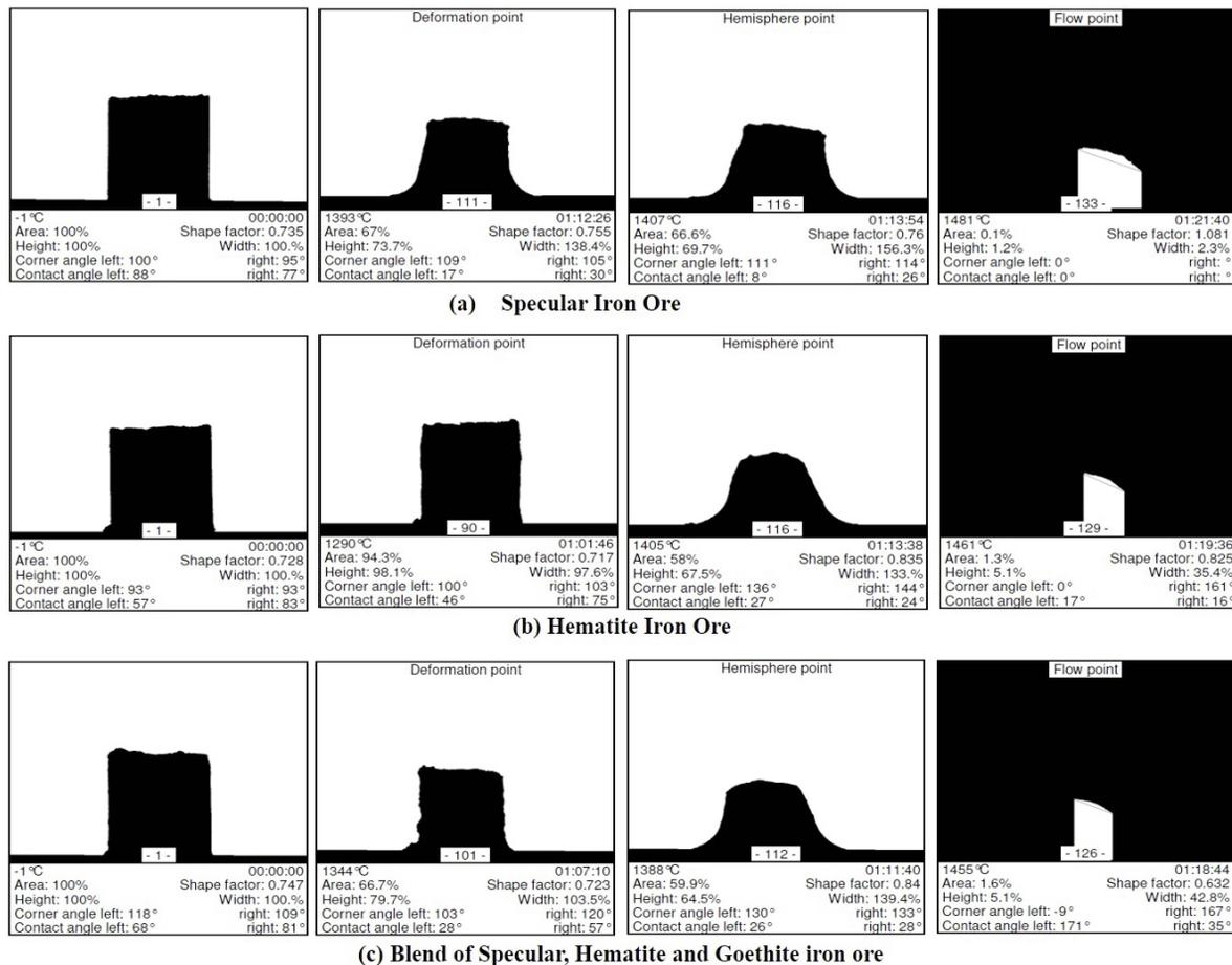
Figure 11. Assimilation behaviour of (a) Specular I/O, (b) Hematite I/O and (c) blend of (Specularite, Hematite and Goethite I/O)
