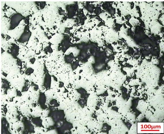
Figure 2. Mineralogy of hematite I/O (100X)
