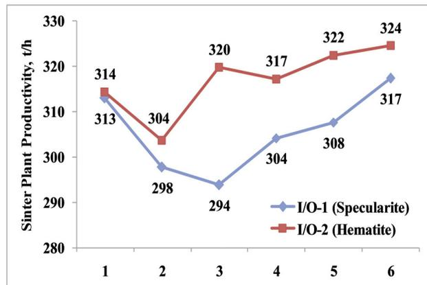
Figure 1. Effect of iron ore type on sinter plant production (t/h, average of 6 consecutive days)
