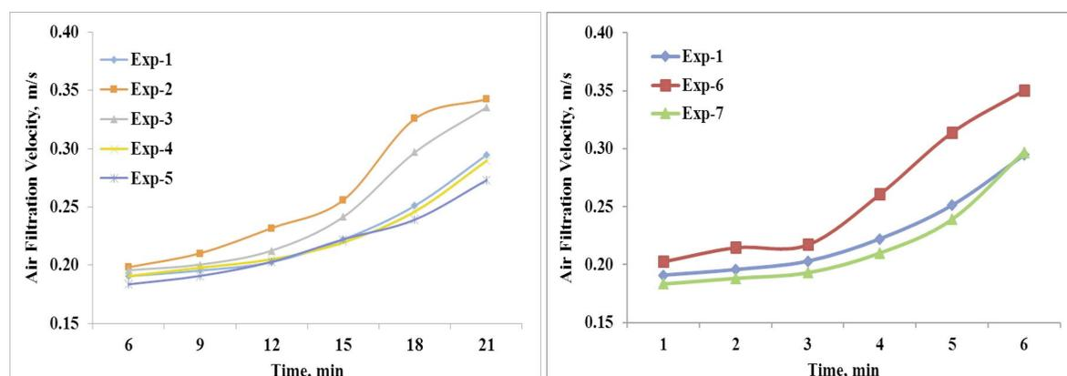
Figure 9. Average air filtration velocity (m/s) of the sintering process at an interval of 3 minutes
