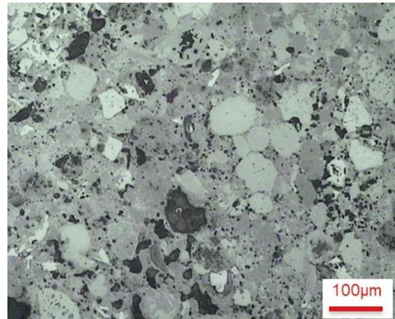
Figure 4. Mineralogy of Goethite iron ore @ 100X magnification
