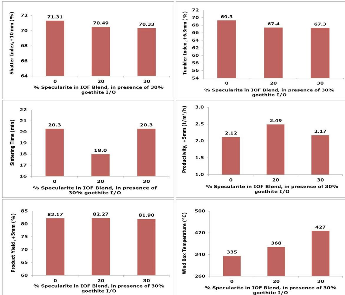
Figure 10. Graphical representation of sintering behaviour and sinter qualities at different combination of experimental trials
