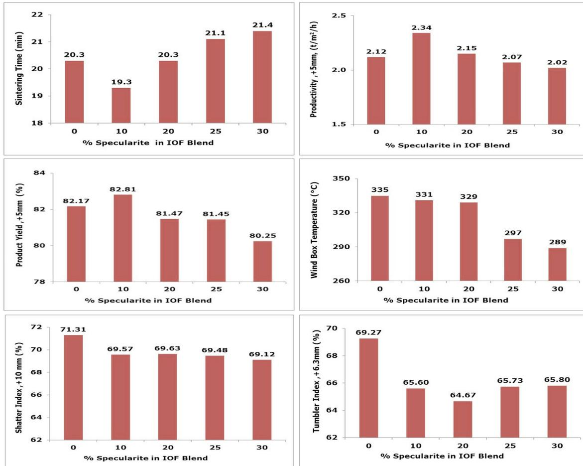
Figure 8. Graphical representation of sintering behaviour and sinter qualities at different combination of experimental trials
