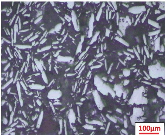
Figure 3. Mineralogy of Specular iron ore @ 100X magnification
