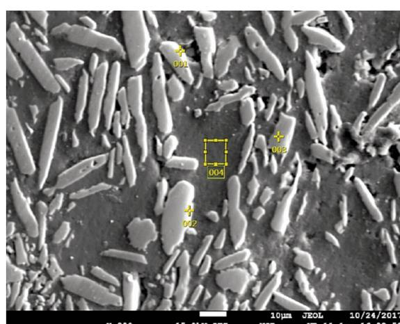
Figure 5. Mineralogy of Specular iron ore @ EPMA (800X magnification)
