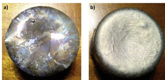
**Figure 6.** (a) Co-W alloy ingot obtained during 3C process; (b) final Co-9Al-9W alloy ingot obtained during 3C process
