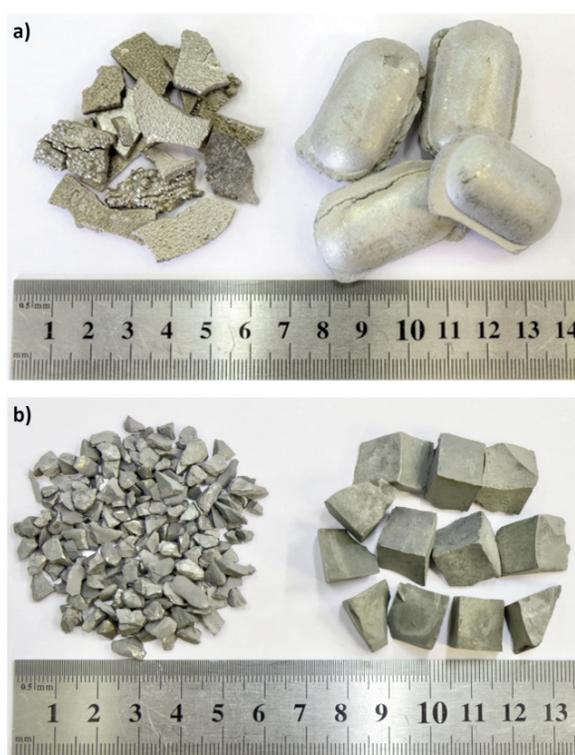
**Figure 1.** Morphology of (a) cobalt feedstock materials used for Co-9Al-9W alloy smelting: electrolytic cobalt (left) and pressed Co pellets (right), and (b) tungsten feedstock materials used for Co-9Al-9W alloy smelting: crushed W pellets (left) and uncrushed W pellets (right)
