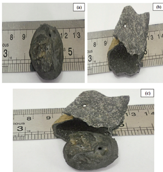
Figure 9. (a) Metallic product (b) Slag and (c) Metallic product and slag before separation
