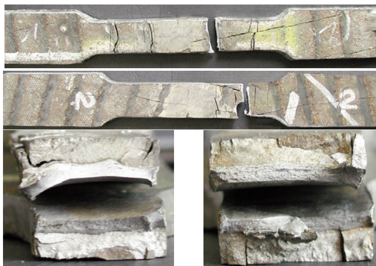
Figure 13. View of welded joints after a tensile test with fractures
