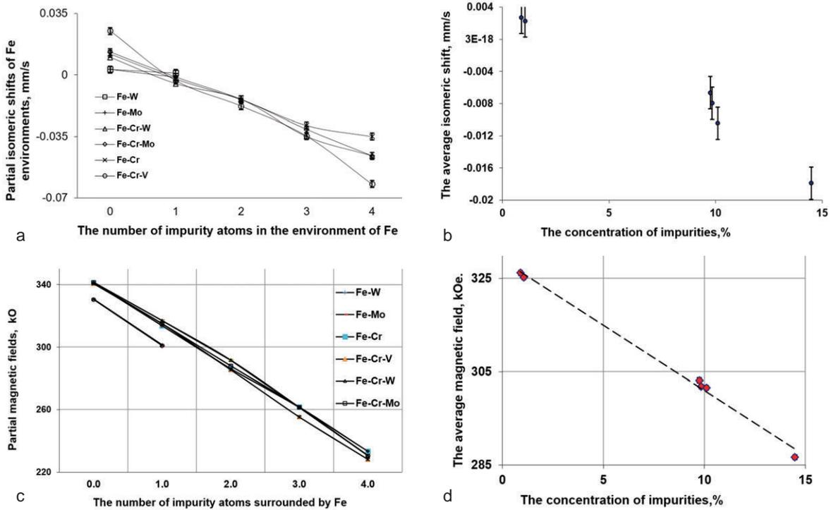
Figure 1. Dependence of partial isomeric shift (a) and partial magnetic field on iron-57(c) on the number of shortest neighbors (SN) and the average values on impurity's concentration (b and d)\*
