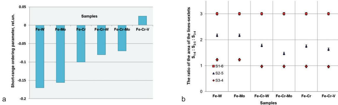
Figure 4. Dependence of the short-range ordering parameter (a) and areas' ratio (b) on the sample content
