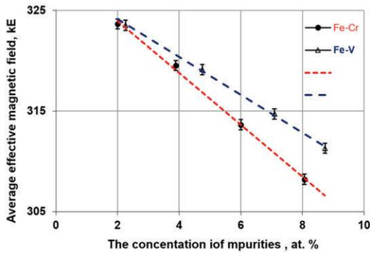
Figure 2. Dependence of itinerant field strength on impurity concentration
