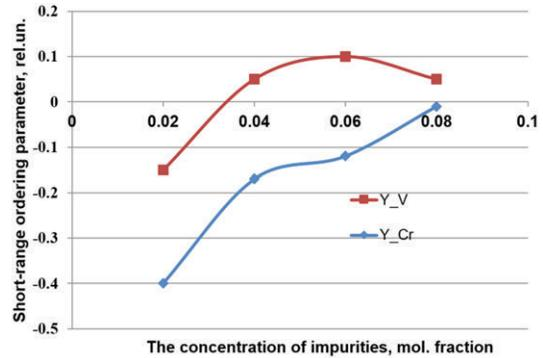
Figure 3. Dependence of the short-range ordering parameter on impurity content
