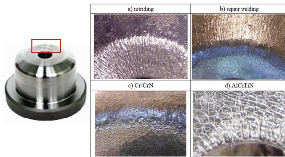
Figure 5. Macro view of the face part of analyzed tools after manufacturing approx. 4000 forgings: a) after nitriding, b) after pad welding, c) with Cr/CrN layer, d) with AlCrTiN layer
