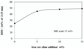
Figure 8. Effect of iron ore slime addition on RDI of mill scale added hematite pellet
