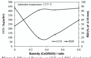
Figure 4. Effect of Basicity on CCS and RDI of indurated fluxed pellet
