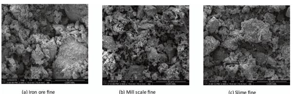
(b) Mill scale fine (c) Slime fine Figure 2. Surface morphology of different fines under SEM microscope
