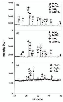
Figure 1. XRD analysis of iron ore, slime and mill scale; (a) iron ore, (b) iron ore slime, (c) mill scale
