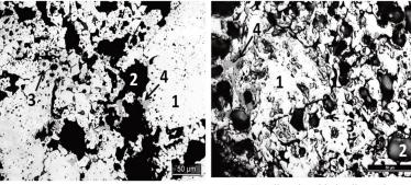
15 wt% mill scale added pellet without slime (Indurated at 1275°C)
