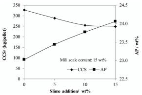
Figure 5. Effect of increasing addition of iron ore slime on the CCS and Apparent Porosity of mill scale containing acidic hematite pellet
