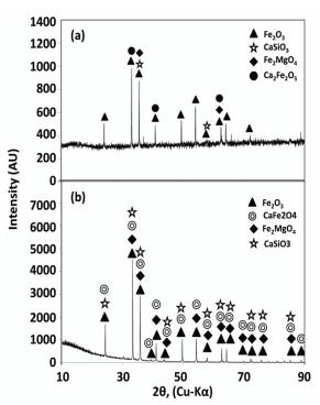
Figure 11. XRD of mill scale added basic pellet (0.3 basicity) with and without the addition of iron ore slime (a) 15 wt% mill scale added pellet without slime (indurated at 1275°C) (b) 15 wt% mill scale added pellet with 15% slime (indurated at 1275°C)
