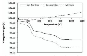
Figure 3. Thermo-gravimetric analysis of several raw materials
