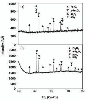
Figure 7. XRD pattern of mill scale added acidic pellet and with and without the addition of iron ore slime (a) Mill scale (15%) added pellet without slime (b) Mill scale (15%) added pellet with 15% slime
