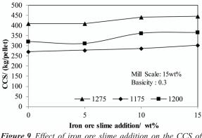
Figure 9. Effect of iron ore slime addition on the CCS of mill scale added basic hematite pellet
