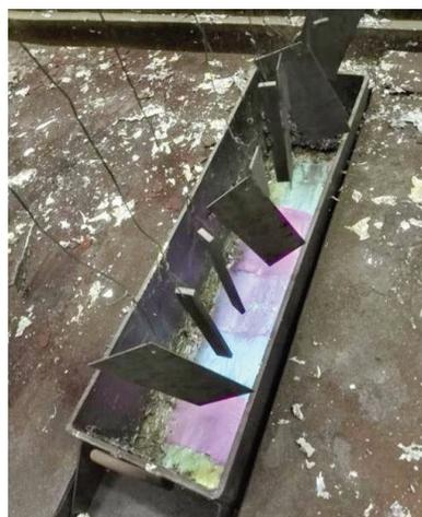
**Figure 3.** Samples hanging from a crane (not shown) above the liquid bath during the pre-heating period before their immersion (one can see the colors on the surface of the bath).
