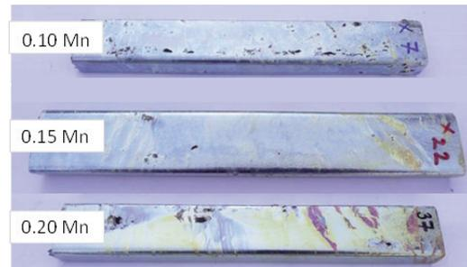
Figure 6. Photos of 40×20×2×250 mm hollow profiles 1 treated in different baths (Mn contents are given in m/m%)
