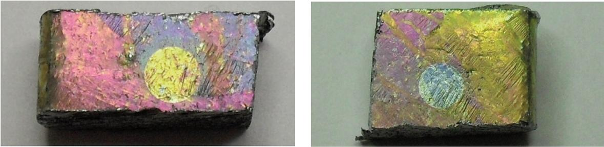
**Figure 16.** Photos of the sputtered by SNMS sample (Fig.10, 0.2 m/m% Mn) for 70 s (left) and for 140 s (right). See the color change in the circular sputtered spots.
