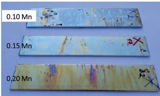
Figure 9. Photos of 50×4×250 mm flat steel 1 samples treated in different baths (Mn contents are given in m/m%)
