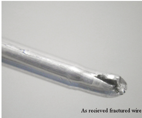
Figure 2. Digital image of fractured EC grade aluminum wire after wire drawing die assembly
