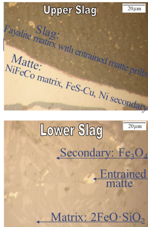
Figure 5. Upper and lower part of converter slag after addition of 5 wt% coke and treatment at 1300 °C for one hour
