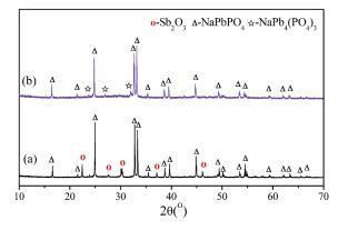
**Figure 8.**XRD patterns of Sb<sub>2</sub>O<sub>3</sub>, PbO and NaPO<sub>3</sub> at different molar ratio(a) PbO:Sb<sub>2</sub>O<sub>3</sub>: NaPO<sub>3</sub>=2:1 :2; (b) PbO:Sb<sub>2</sub>O<sub>3</sub>:NaPO<sub>3</sub>=2:1:4;
