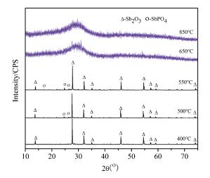
Figure 3. XRD patterns of Sb<sub>2</sub>O<sub>3</sub> and NaPO<sub>3</sub> mixture at different temperature (a)-803K;(b)-923K;(c)-1123K
