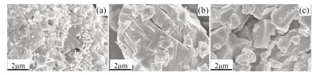
Figure 4. SEM images of Sb<sub>2</sub>O<sub>3</sub> and NaPO<sub>3</sub> mixture at different temperature (a)-803K; (b)-923K; (c)-1123K
