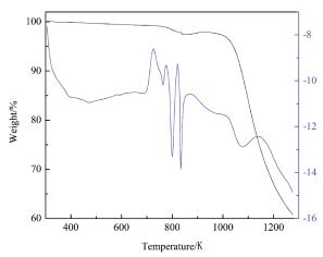
Figure 2. TG-DSC pattern of Sb<sub>2</sub>O<sub>3</sub> and NaPO<sub>3</sub> mixture
