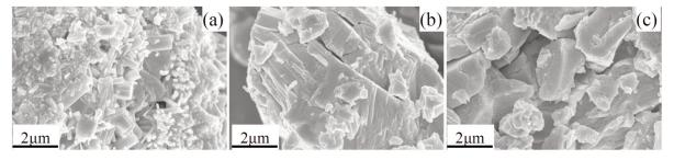
Figure 7. SEM images of PbO and NaPO<sub>3</sub> at different temperature(a)-923K;(b)-1023K;(c)-1123K
