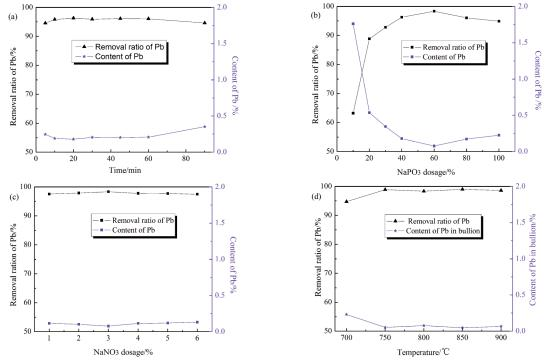
**Figure 9.** Effects of (a) reaction time, (b) dosage of  $NaPO_3$ , (c) dosage of  $NaNO_3$ , (d) reaction temperature on removal ratio of lead and content of lead in bullion
