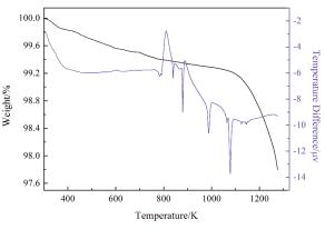
Figure 5. TG-DSC pattern of PbO and NaPO<sub>3</sub>
