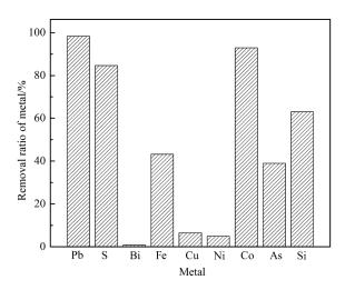
Figure10. Removal ratio of various impurity metals in the refining process
