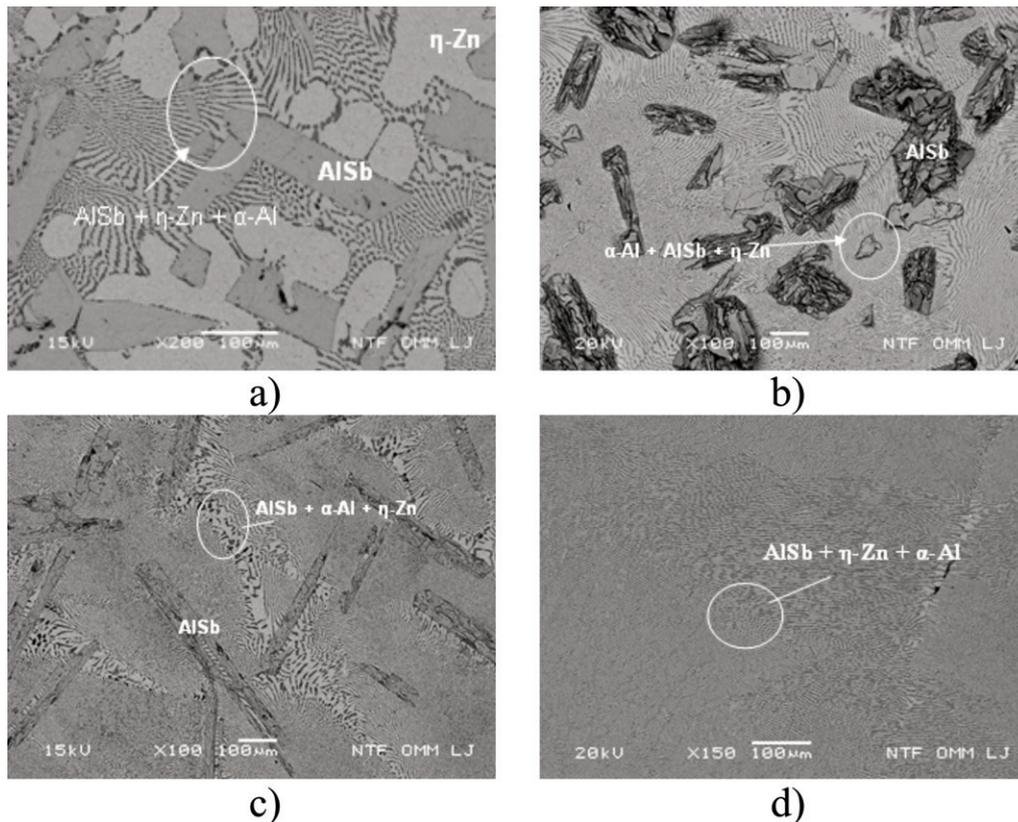
Figure 4. Microphotographs of selected samples in Zn-rich corner:
