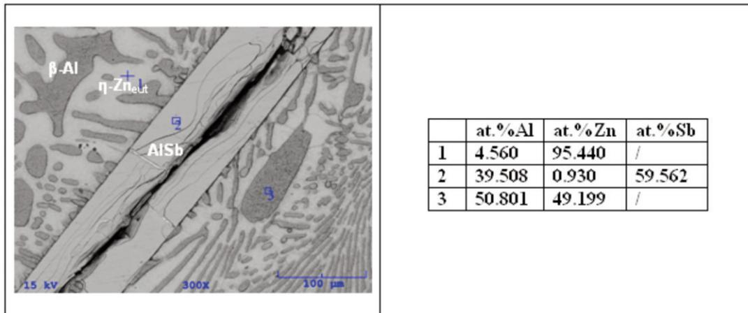
Figure 1. BSE micrograph of AZS4 homogenized at 330 °C for 10 days
