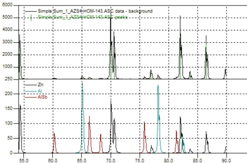
Figure 2. XRD pattern of the sample homogenized AZS4
