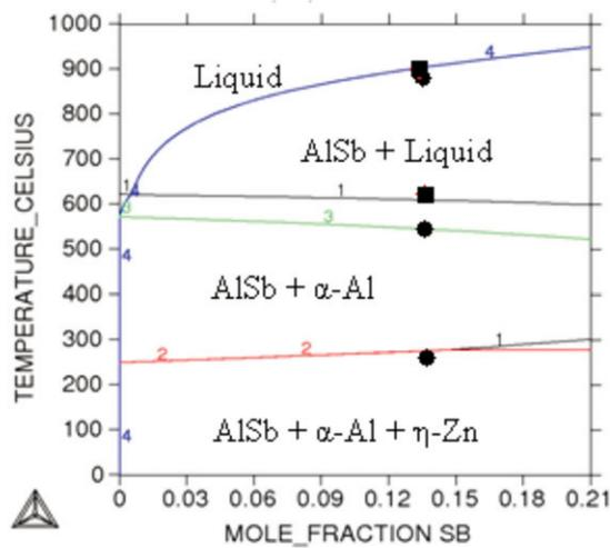
Figure 11. Isolethe phase diagram of AZS13: ● heating, ■ cooling
