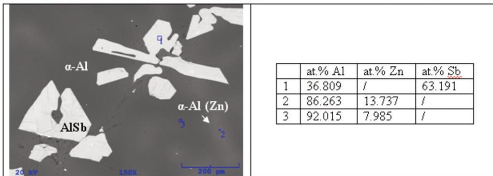
Figure 10. Microphotograph of AZS 13 with related EDS analysis
