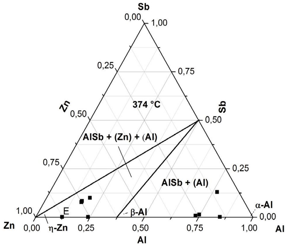
Figure 12. The 374 °C isothermal section with compositions of alloys
