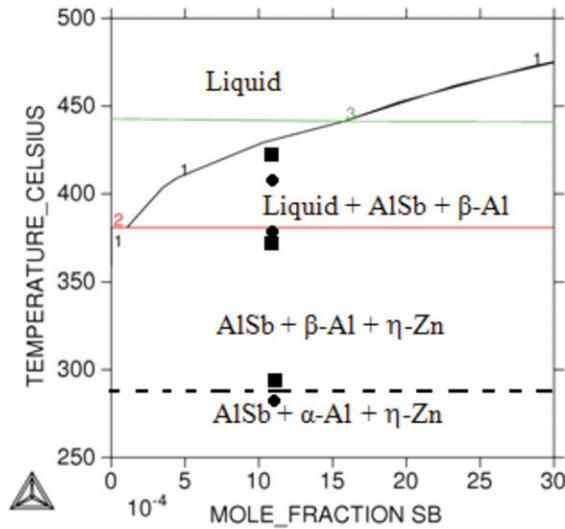
Figure 9. Isopleth phase diagram of AZS11: - - experimental, — predicted, • cooling, ■ heating
