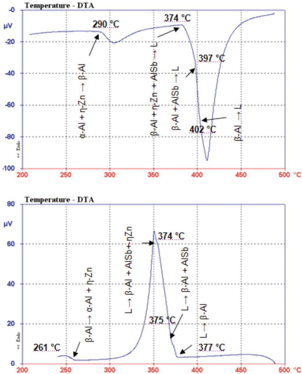
Figure 6. DTA heating and cooling curve of AZS 11
