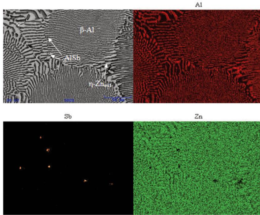
Figure 7. Elemental mapping of sample AZS11
