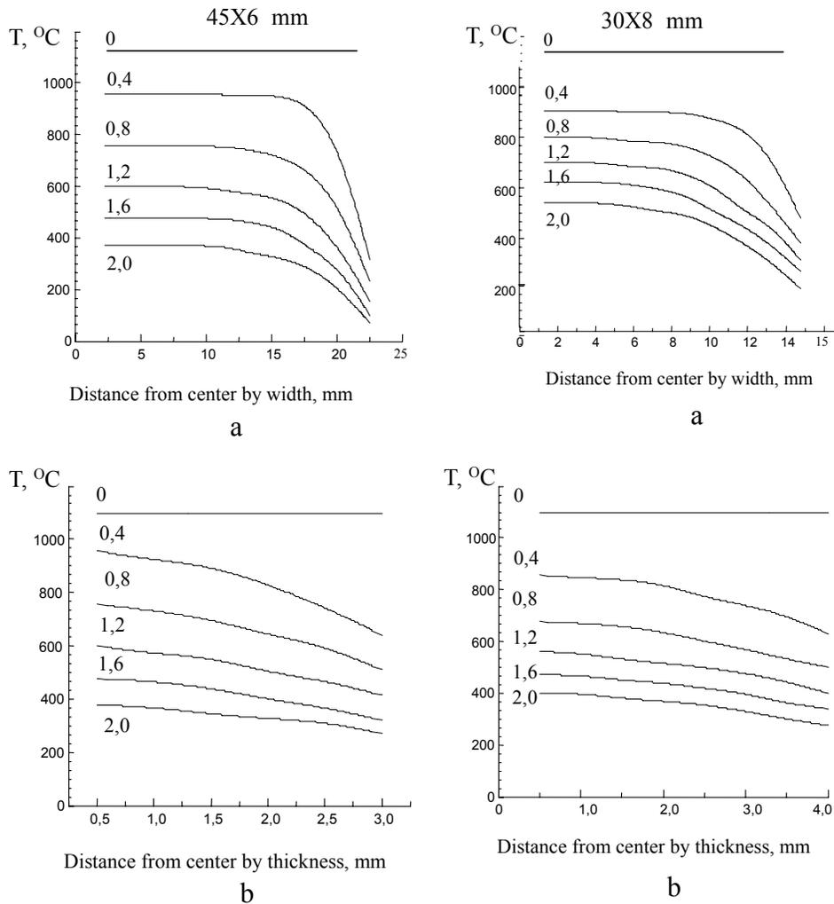
Fig. 1. Temperature distribution along the width (a) and thickness (b) of stripe rolled steel (cross-section 45x6 and 30x8 mm) under accelerated cooling [ $\alpha = 10$  kW/m<sup>2</sup>k]; figures near the curves - time since the beginning of the transformation, s; a - distance from the centre considering the width; b - distance from the centre considering the thickness.
