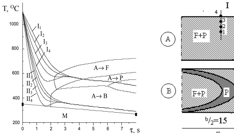
Fig. 2. The scheme of stripe rolled steel structure forming with the cross-section 30x8 mm with different cooling intensities (according to the results of the calculation): A - heat irradiations ratio  $\alpha = 7 \text{ kW/m}^2\text{K}$ ; B -  $\alpha = 10 \text{ kW/m}^2\text{K}$
