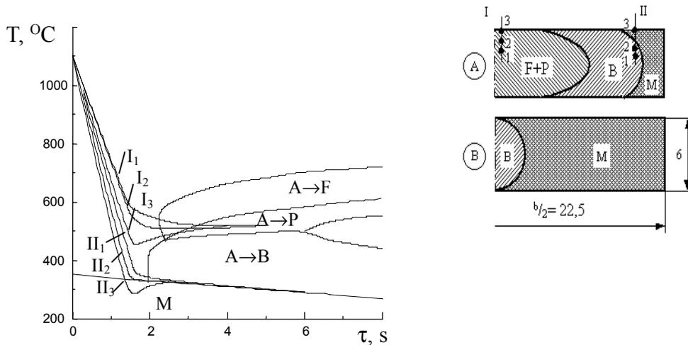
Fig.3. The scheme of stripe rolled steel structure forming with the cross-section 45x6 mm with different cooling intensities (according to the results of the calculation): A - heat irradiations ratio  $\alpha = 7 \text{ kW/m}^2\text{K}$ ; B -  $\alpha = 10 \text{ kW/m}^2\text{K}$ .
