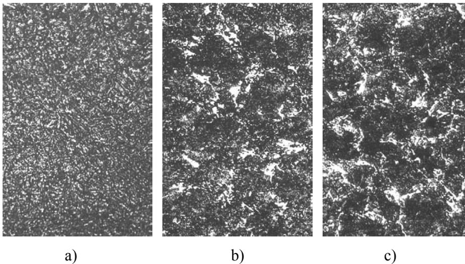
*Fig. 4. The structure of the stripe of cross-section 45x6 mm made of low-carbon steel after the accelerated cooling in the mill flow: a - the section, adjoining the upper and lower parts of the stripe; b - transitional layer; c - central part of the cross-section of the stripe. Enlargement 400:1*
