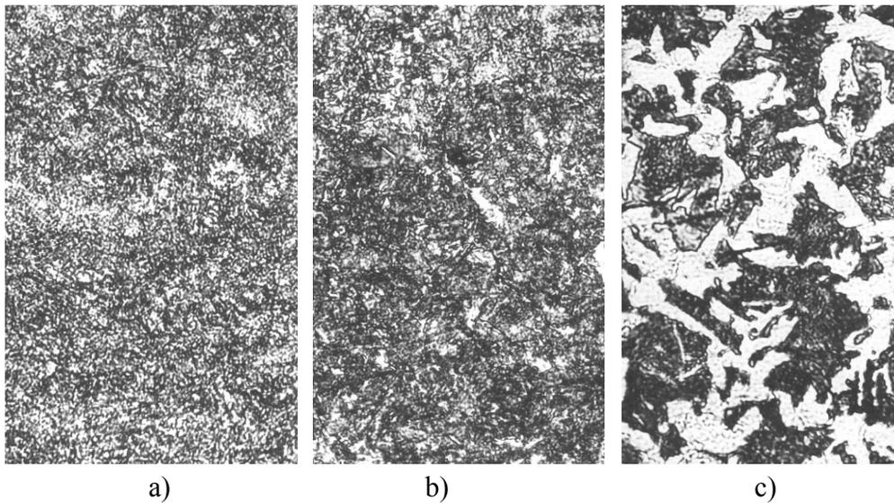
*Fig. 5. The structure of the stripe of cross-section of 45x6 mm made of low-carbon steel in hot-rolled condition: a - buttend of the stripe (the edge); b - transitional layer (4-8 mm of the buttend); c - central part. Enlargement 400:1*
