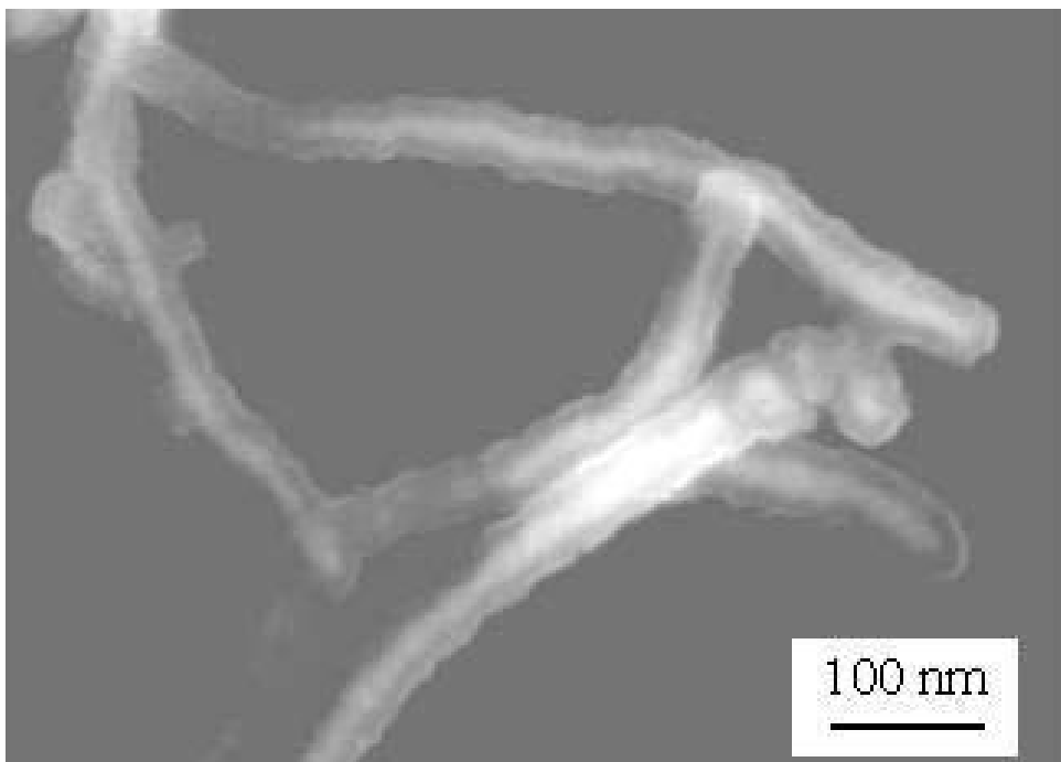
Figure 10. An SEM image of tin filled CNTs produced similarly as those shown in Figure 9b, but the electrolysis was on a much greater scale.
