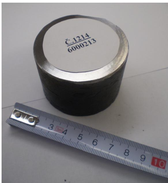
Fig. 1. The cylindrical steel samples for the laboratory analysis by g-spectrometry
