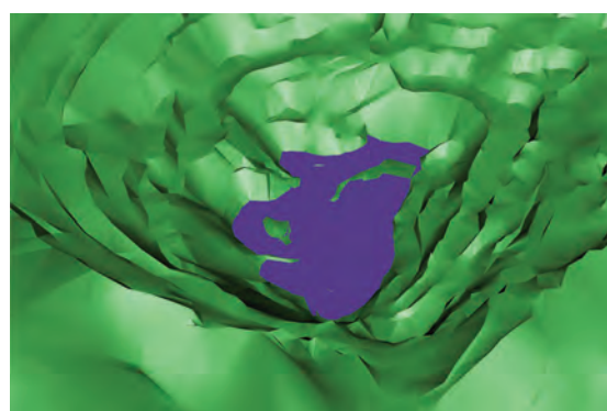
Fig. 4. Water accumulation on the bottom of the open pit Cerovo
