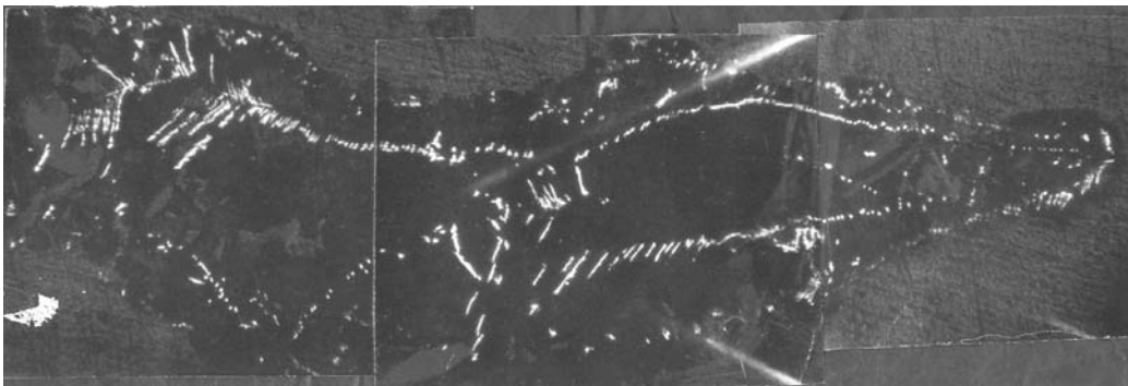
Figure 2. A longitudinal section of the fibrous deposit. The lower end of the bunch, magnification - 112 times.
