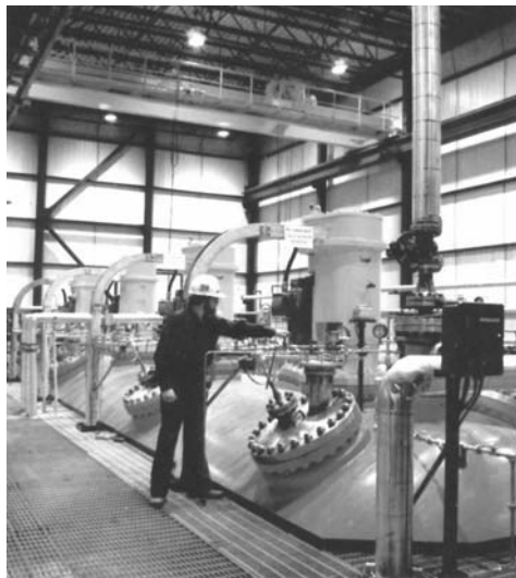
Figure 8. Pressure leaching of zinc sulfide concentrates in dilute sulfuric acid at 150° C and under oxygen pressure
