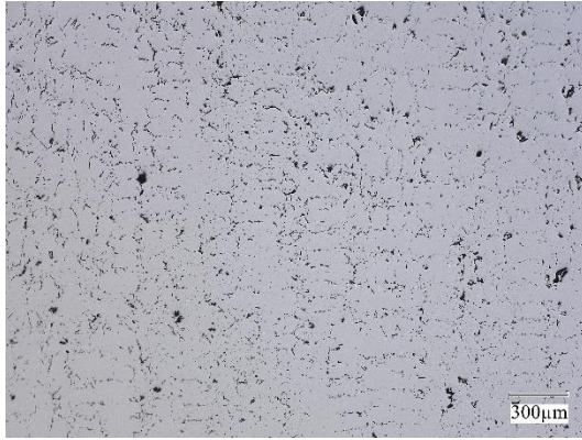
Figure 12. Unidirectional structure, a) v = 2,50 * 10^{-6} \text{ m/s} ; b) v = 2,50 * 10^{-6} \text{ m/s} , etched with Nital; c) v = 5,56 * 10^{-6} \text{ m/s} ; d) v = 5,56 * 10^{-6} \text{ m/s} , etched with Nital; e) v = 8,33 * 10^{-6} \text{ m/s} ; f) v = 8,33 * 10^{-6} \text{ m/s} , etched with Nital; g) v = 1,11 * 10^{-5} \text{ m/s} ; h) v = 1,11 * 10^{-5} \text{ m/s} , etched with Nital
