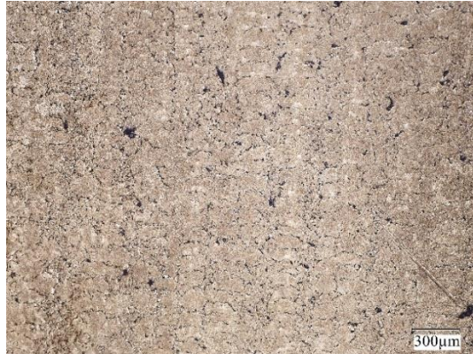
Figure 12. Unidirectional structure, a) v = 2,50 * 10^{-6} \text{ m/s} ; b) v = 2,50 * 10^{-6} \text{ m/s} , etched with Nital; c) v = 5,56 * 10^{-6} \text{ m/s} ; d) v = 5,56 * 10^{-6} \text{ m/s} , etched with Nital; e) v = 8,33 * 10^{-6} \text{ m/s} ; f) v = 8,33 * 10^{-6} \text{ m/s} , etched with Nital; g) v = 1,11 * 10^{-5} \text{ m/s} ; h) v = 1,11 * 10^{-5} \text{ m/s} , etched with Nital
