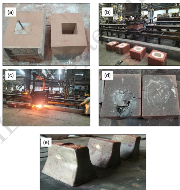
Figure 1- Fabrication sequence and geometry of the Y-block castings used in the present investigation: (a) preparation of the sand mould with Y-block cavity dimensions, (b) mould arrangement before pouring (c) molten metal pouring into the mould cavity (d) solidified Y-block castings after shakeout, and (e) ASTM A532 Y-block specimens used for heat treatment and characterization.
