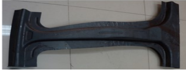
Figure.3: Warm stamped B-pillars from medium-Mn steel [4]
