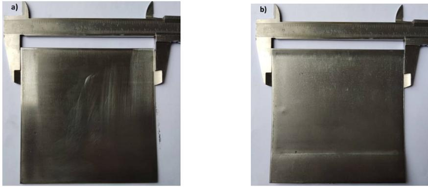
**Fig 2** DC04 steel sheet a) before ECAP, b) S1 after ECAP
