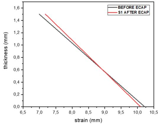
**Fig. 19** The true strain/thickness graph for sheet before ECAP and S1 after ECAP
