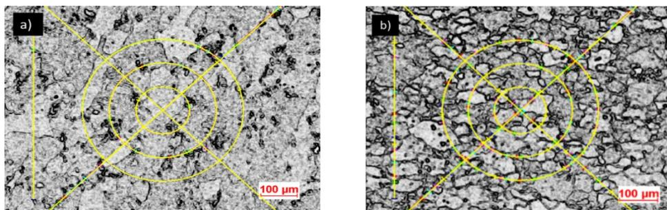
**Fig. 11** Intercept method (x100): a) before ECAP; b) S1 after ECAP.
