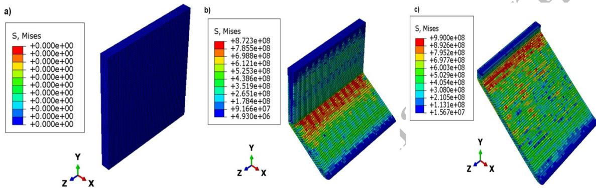
**Fig. 8** ECAP simulation of DC04 sheets: a) initial state, b) middle of the simulation, c) end of the simulation.
