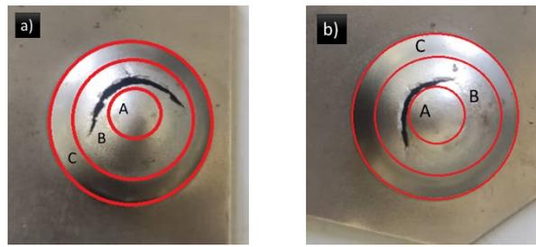
**Fig. 17** different deformation zones that the sheets underwent after the Erichsen tests: a) before ECAP, b) S1 after ECAP.
