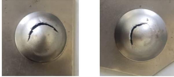
**Fig. 16** Plate cracking after Erichsen test: a) before ECAP; b) after ECAP
