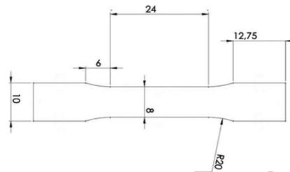
Fig. 5 Tensile test specimen according to EN ISO 6892-1.
