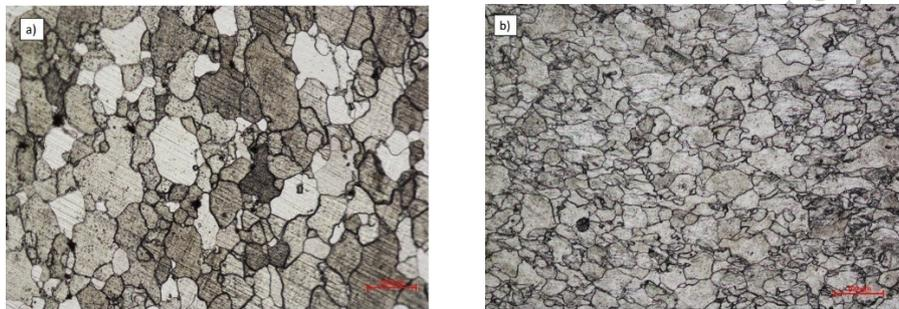
**Fig. 10** Microstructure of the sheet (x100): a) before ECAP; b) S1 after ECAP.
