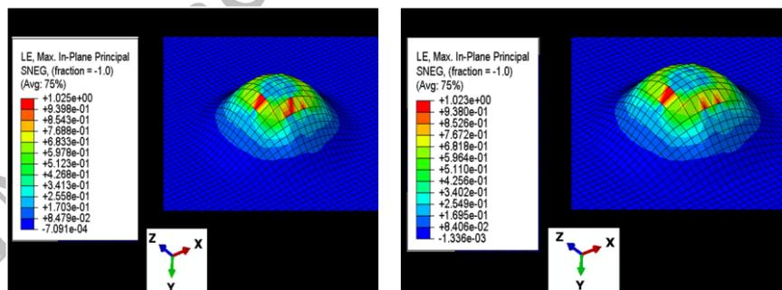
**Fig. 18** simulation of the Erichsen tests of sheets: a) before ECAP, b) S1 after ECAP
