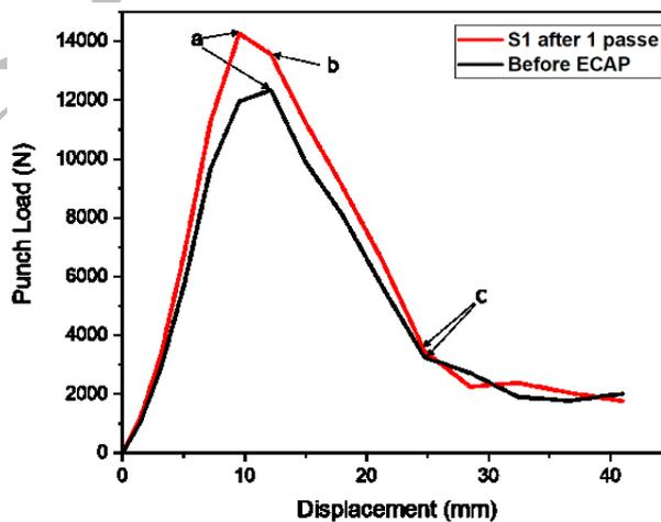
**Fig. 20** representation of the punch load (N)-Displacement (mm) curve.
