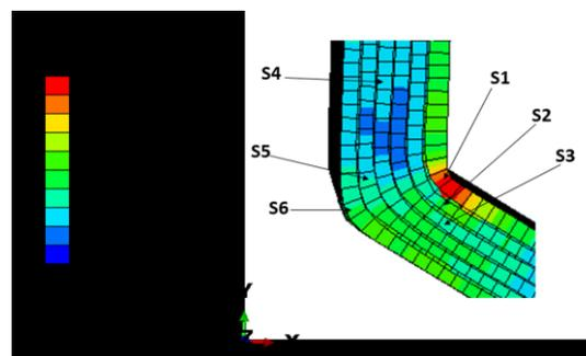
**Fig. 9** distribution of stress of V. Mises during the simulation.
