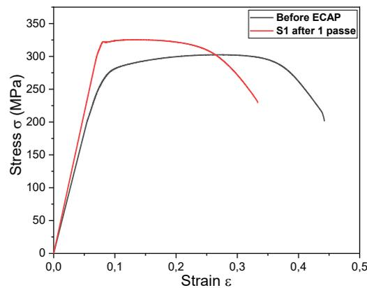
**Fig. 14** Strain-stress curves before and after ECAP for S1.
