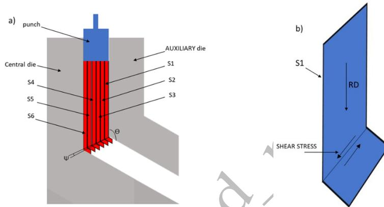
**Fig. 3** a) schematic diagram of the ECAP process. b) rolling direction (RD) versus metal flow in ECAP
