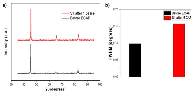
**Fig. 13** a) X-ray diffraction patterns before and after ECAP; b) FWHM values.
