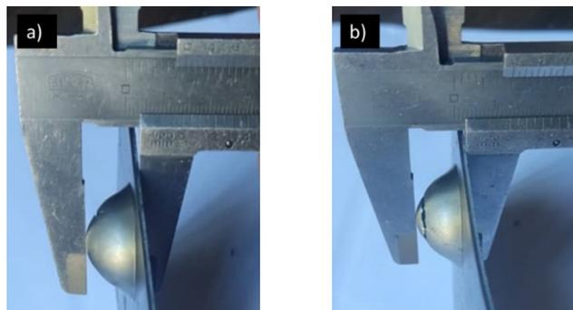
**Fig. 15** Method of measuring the deformation depth of the cup: a) before ECAP; b) after ECAP.
