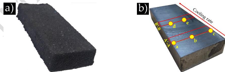
Figure 2. Plate thickness of 12.7 mm a) surface in contact with green sand, and b) plate rectified.
