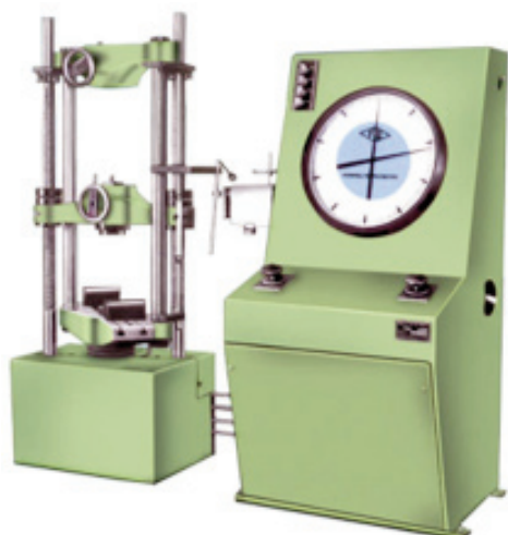
Figure S1. Universal testing machine used for tensile testing. ASI UTM Machine 60 Tonnes
