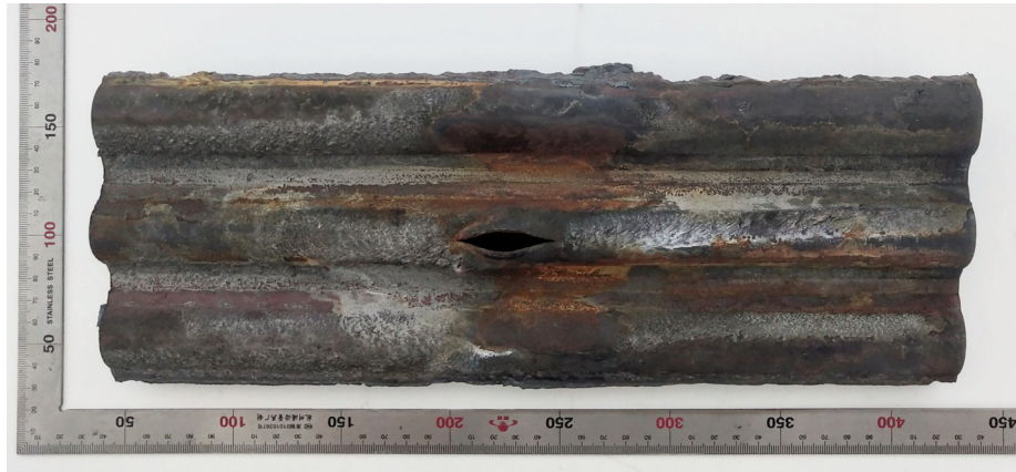
Figure 1. The damaged superheater tube received for failure analysis
