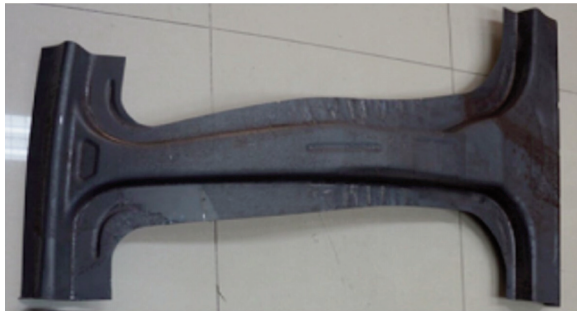
Figure 3. Warm stamped B-pillars from medium-Mn steel recently developed [6]
