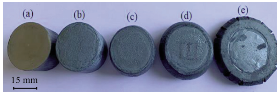
Figure 4. Produced samples a) sintered, b) homogenized, c) 20%, d) 40% and e) 60% deformed
