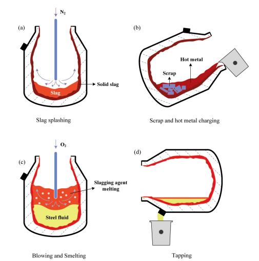
Figure 1. Flow chart of steelmaking process in BOF. a Slag splashing; b Scrap and hot metal charging; c Blowing and smelting; d Tapping
