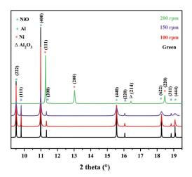
Figure 5. XRD patterns of pure and milled powders during 1.5 hour using a BPR of 42:1 for different milling speed 100,150 and 200 rpm
