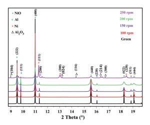
Figure 2. XRD plots of specimens milled for 1 hour as a function of milling speed (100,150,200 and 250 rpm) with a BPR of 42:1
