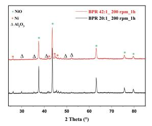
**Figure 9.** XRD patterns of milled and sintered samples at 800°C for 2 hours
