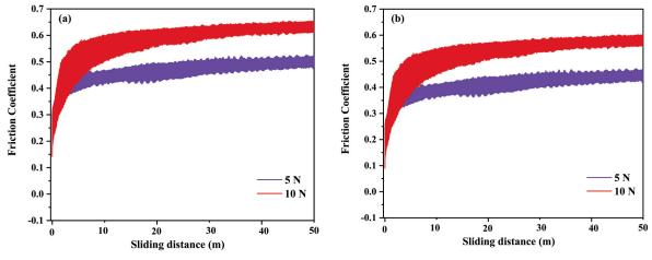
Figure 13. Impact of applied forces (5 and 10 N) on the friction coefficient of sintered specimens, (a) unmilled sample and (b) a sample milled with a BPR of 42:1 at 200 rpm for 1 hour and subsequently sintered at 1100 °C
