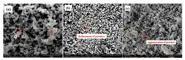
Figure 6. SEM micrographs of unmilled and milled samples with a rotation speed of 200 rpm for 1 hour (a) unmilled (b) BPR 20:1 (c) BPR 42:1
