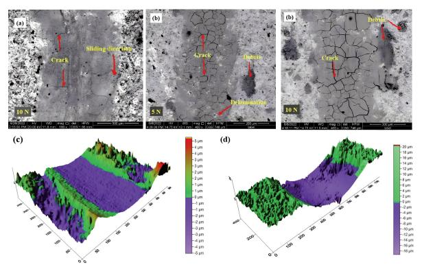
Figure 14. SEM images and 3D morphologies of worm surfaces (a) unmilled (10N), (b) milled with a BPR of 42:1 at 200 rpm for 1 hour (5 and 10 N),(c) 3D of the unmilled sample at 10N and (d) 3D milled sample at 10 N
