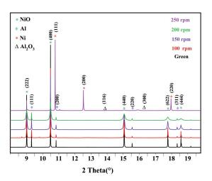
Figure 1. XRD plots of pure and milled NiO/Al powder mixture with a BPR of 20:1 milled for 1 hour as a function of milling speed 100,150,200 and 250 rpm
