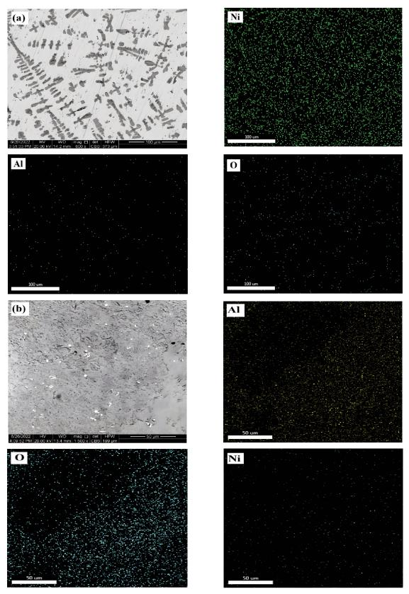
Figure 12. SEM images and EDS mapping of sintered sample at 1100°C for 2 hours (a) Nickel phase and (b) Alumina phase
