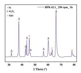
**Figure 10.** XRD profile of milled and sintered sample at 1100°C for 2 hours
