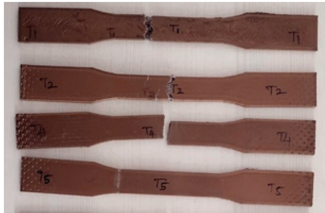
Figure 6. Fractured tensile test sample
