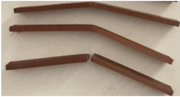
Figure 9. Fractured flexural test sample
