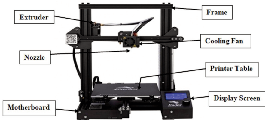
Figure 2. Setup of FDM machine
