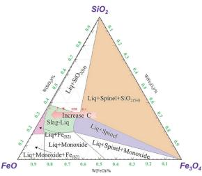
Figure 5. Ternary diagram of SiO<sub>2</sub>-FeO-Fe<sub>3</sub>O<sub>4</sub> at 1250 °C
